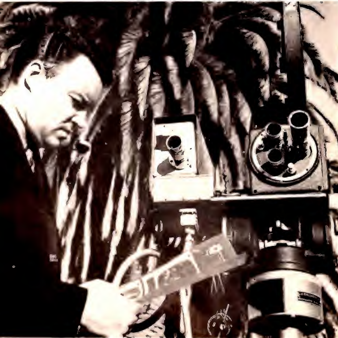
Snazelle stands beside two-headed dolly where movie camera (r) shoots scene as the closed circuit tv camera (l) helps monitor its direction.
