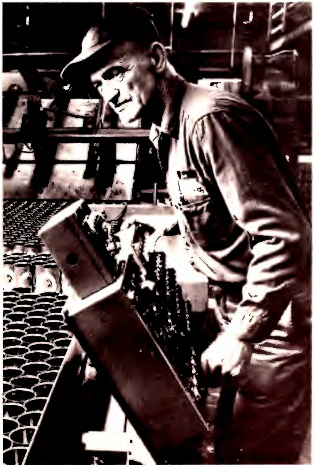
Four lines feed 1,000 empty cans per minute.
