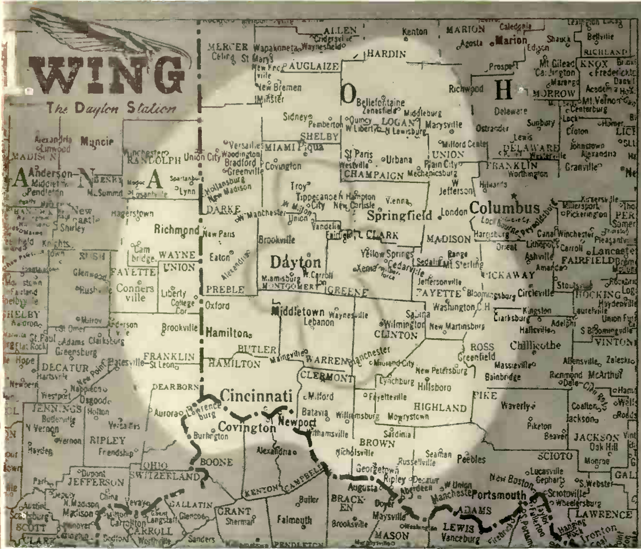
MAP KEY: Daytime coverage: large unshaded area. Nighttime coverage: smaller, outlined area
