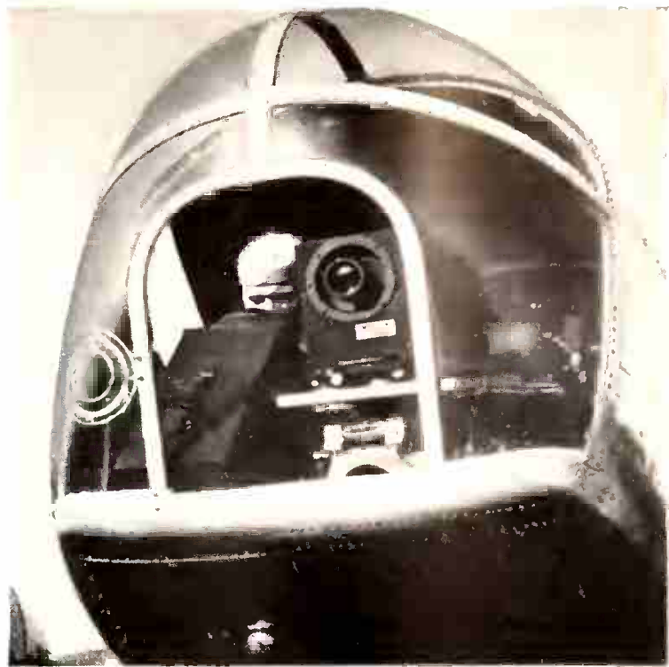
Mounted in the nose of an airplane, special RCA airborne television equipment will give ground observers a sharp, clear, bird's-eye view of land and sea.
