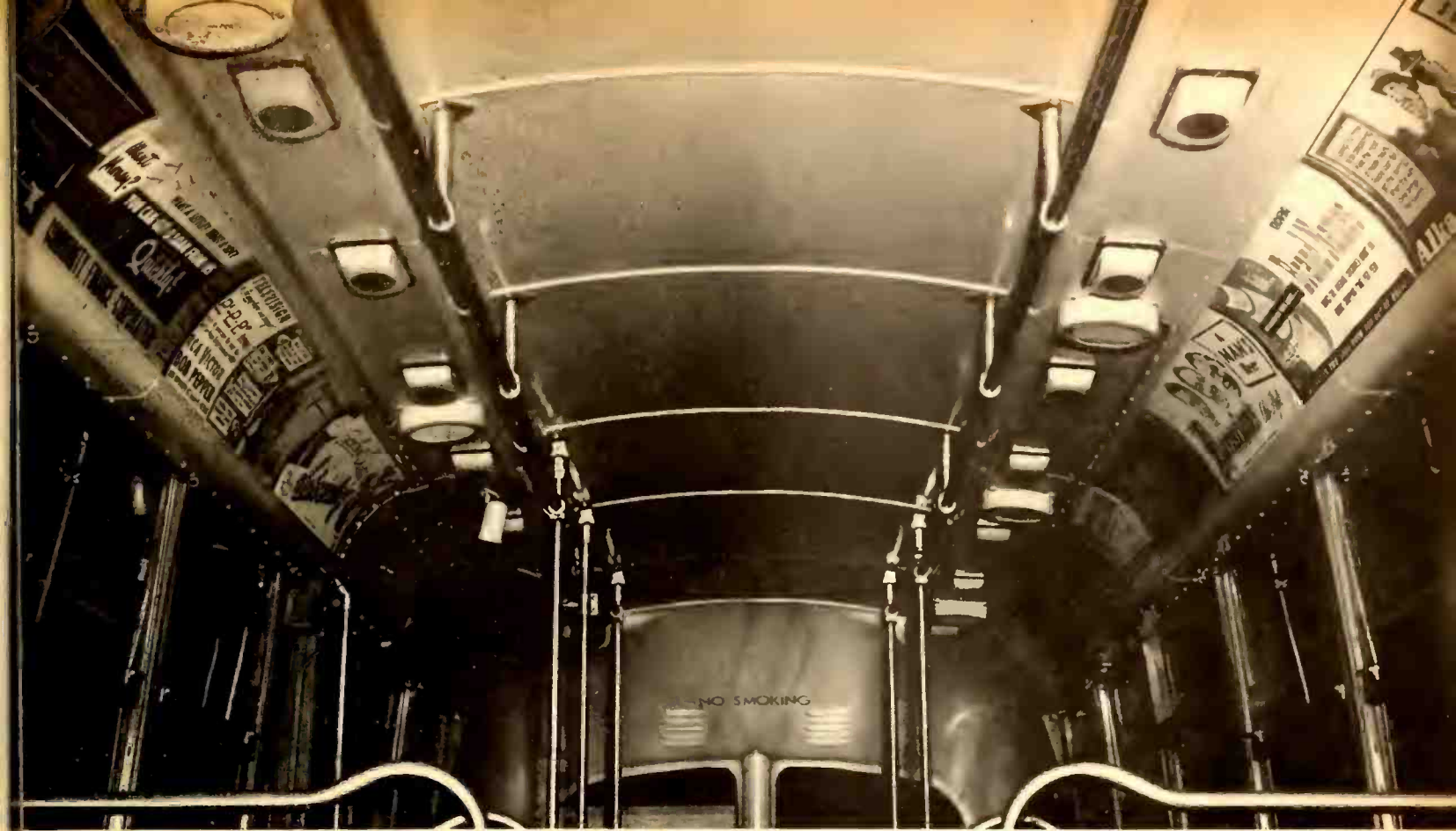
In a transiradio installation one speaker usually alternates between two lights to bring riders an equal volume of sound without blasting at any point
