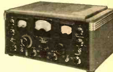
New 1941 Super Skyrider Model SX-28. Sets a new high in quality performance. 15 tubes; Two stages preselection; 80/40/20/10 meter amateur bands calibrated; 6 step wide range variable selectivity; Calibrated bandspread inertia controlled; Frequency coverage 550 kc. to 42 mc. With Crystal and Tubes $15950
