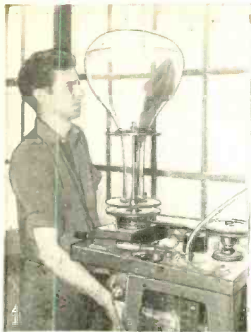
1 Trimming the chemical screen deposited on the inside of glass blank for cathode-ray tube.
