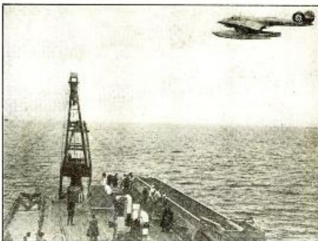
The deck of the first airplane-hotel ship, with large crane for raising plane from water. Note the catapult at the right.
