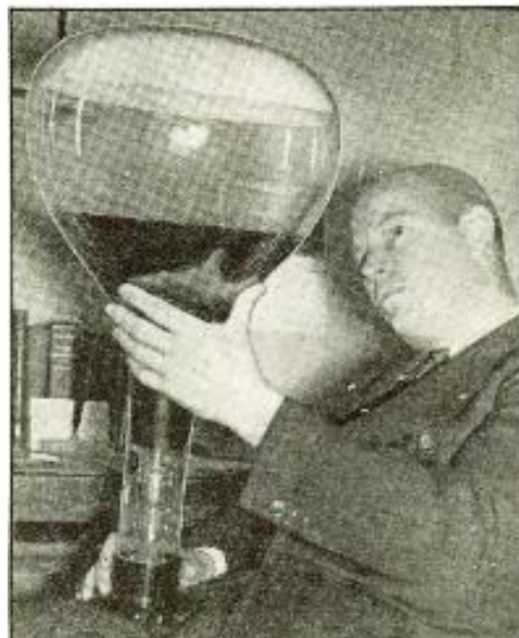
One of the new 12" cathode ray television tubes. (No. 686)
