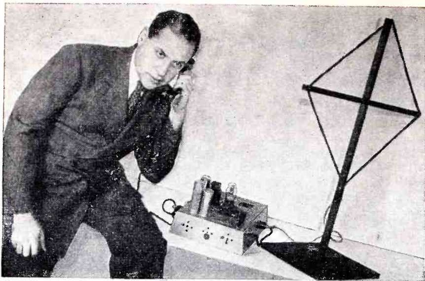
The induction phone transmitter with 1-stage A.F. amplifier, the second tube being a rectifier. Only the mike on the handset is being used in this case.
