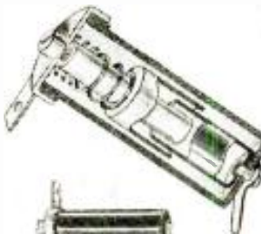
Midget Trimmer, H62. How it works is clearly shown in the above drawing.
