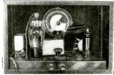
A peek at the chassis of the 2-tube 9\frac{1}{2} to 2,000 meter receiver. (No. 560.)
