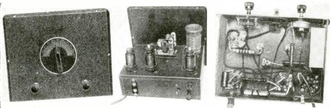
The three photos above show front, rear, and bottom views of the pre-selector here described by Mr. Cisin.
