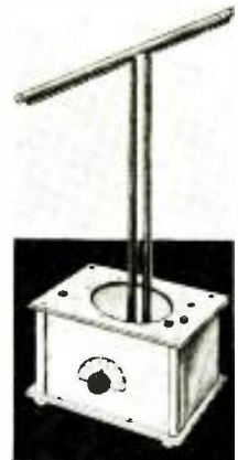
Fig. 7—At left above is shown one form of special antenna used; A is the free upper end, and E is coupled to the transmitter. Fig. 4 at right shows dipole antenna used on one form of 400 mc. transmitter.
