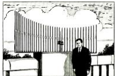
Fig. 6—Portable beam antenna of parabolic shape used by HB9RDL. The chord of the parabola is 3 meters.
