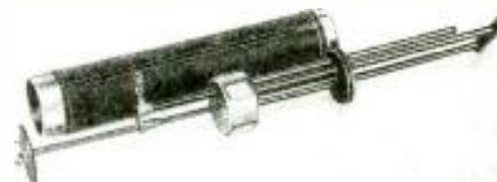
Photo above shows the new ultra short-wave tuning device which employs sliding brass tubes, instead of the familiar copper wire coils. Right—Close-up view of one of the concentric "resonant line" tuners, showing plunger and sliding antenna input terminal. Left—Assembled four-stage concentric line tuner; each circuit can be separately tuned.
