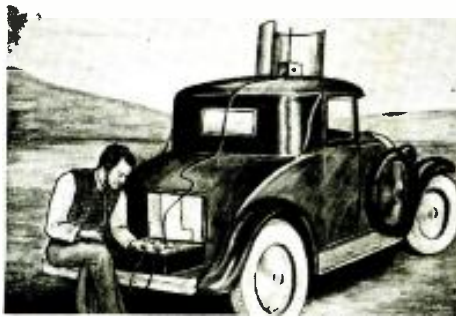
Fig. 5—400 mc. set in use as a "portable" on a car, with antenna arranged in a parabolic reflector.
