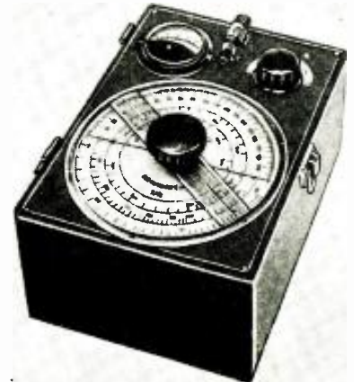
A recent type of German frequency meter having a range of 150 kc. to 60 mc.
