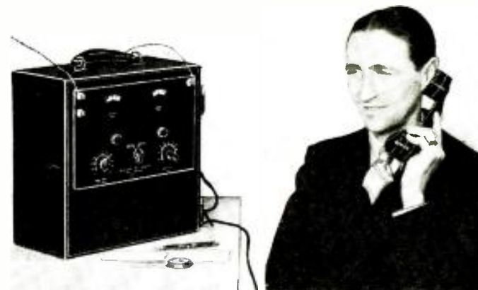
Above—The "Transceptor"—a new 5-meter transmitter-receiver of the portable type shown in use by Mr. Lester. Photos at right show set closed up and below—a rear view, revealing the chassis. No. 544
