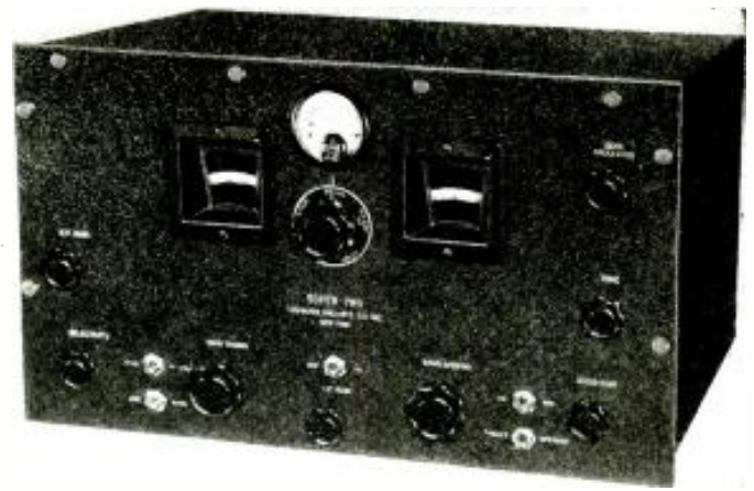
Front view of the Hammarlund "Super Pro" receiver which has a range of 20 mc. to 540 kc. (15 to 555 meters.)
