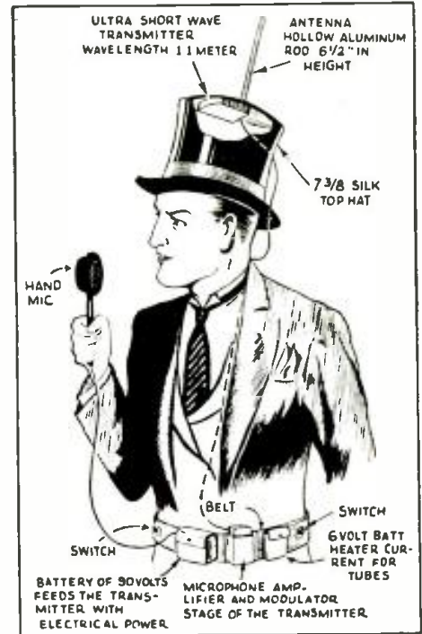
This diagram shows the various component parts of the 1-meter transmitter, the batteries for operating it being carried on a belt around the waist.
