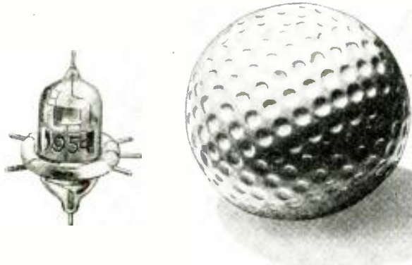
The extremely small size of the new "Acorn"-pentode 954 tube may be judged by comparison with the golf ball at the right of the photo. No. 285.
