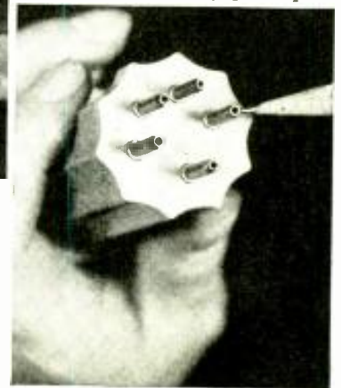
Above: Inserting the "range" disc, after the wavelengths have been properly written in. Right: the large openings in the pins, where the coil winding leads enter and are soldered.
