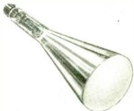
Top photo—front view of the combined "image and sound" television receiver for the Home. Center—rear view of the Loewe "home" televisor, and lower photo the cathode-ray or Braun tube used to reconstruct the image.
