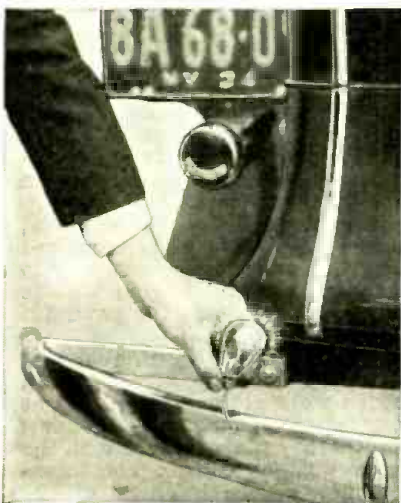
The rear bumper of the new G.E. Police car acts as the "aerial" and is insulated from the body of the car. The power of the charged antenna is shown by the 15-watt lamp, which is here shown lighted on one wire only.
