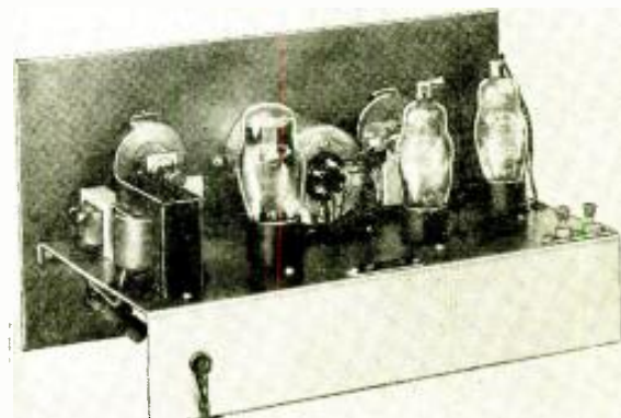
Two photos at the right show front and rear views of the Universal Mascot-3 S.W. receiver. The coils plug-in through the front of the panel and are enclosed in protective insulating shells. (No. 209.)
