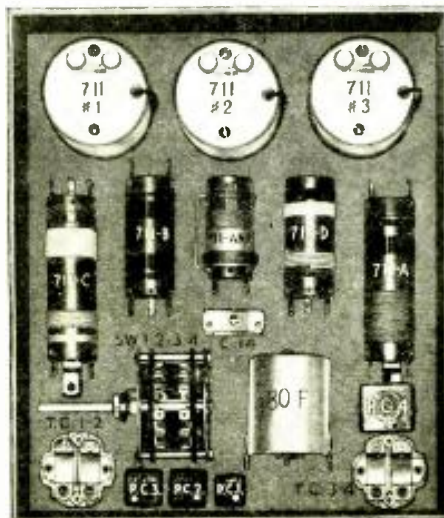
Coil and Band-Switch "kit" for Super-Het, which also includes "I.F." transformers and padding condensers.
