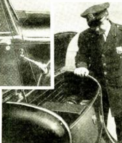
Right—Police officer inspecting the short-wave radio transmitter which is installed in the rear trunk of the car. Tests demonstrated excellent two-way conversation possible.
