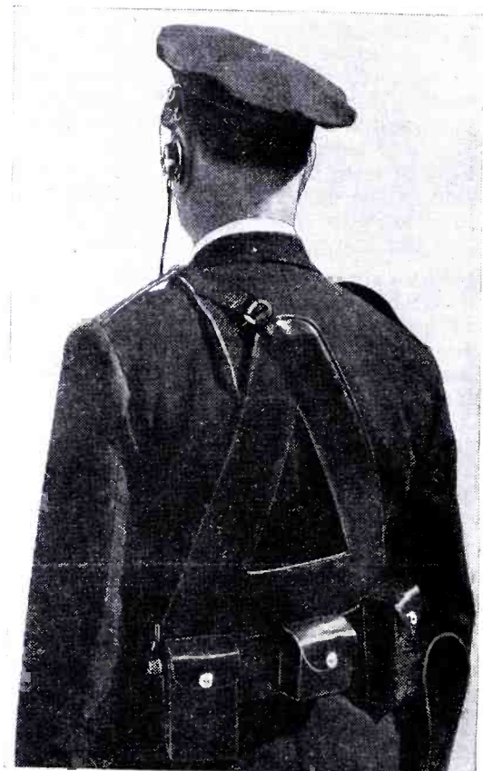
Here's the very latest style in short-wave receivers for the police force—the batteries are carried in the leather pockets on the belt.
