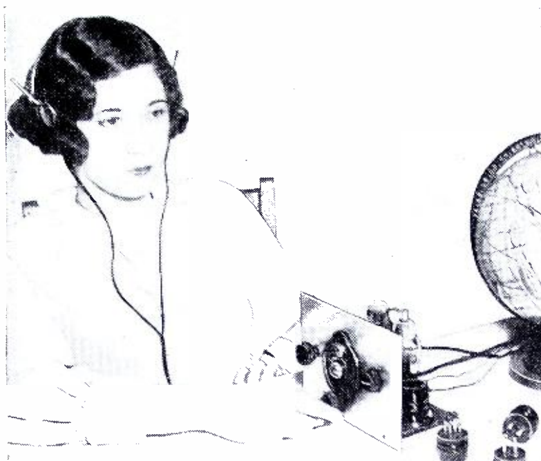
Tuning in European symphony orchestras and vocal programs is a cinch with this very smooth working 2-tube receiver, which is intended for headphone reception.
