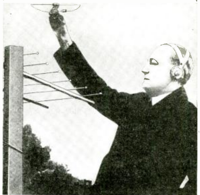
This photo shows Senator Marconi holding a resonance indicator in his hand, in proximity to one of his new ultra short-wave antennas, used in his experiments in Italy.
