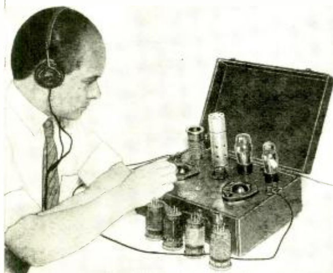
Above—C. W. Palmer, author of the accompanying article making actual test with the Powertone portable 110-volt, A.C.-D.C. Receiver. (No. 116)
