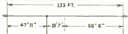
Diagram of typical antenna for 3575 kc. Ant. of No. 14 solid enamelled copper feeder of heavy rubber covered lead-in wire. Use good insulators. Solder feeder on carefully. Feeder at right angles to flat top for first 30% of distance.
