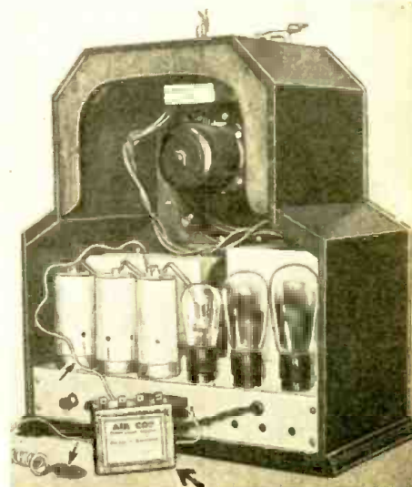
The "police-call" auxiliary tuning device connected to a midget "broadcast" receiver. (No. 102)
