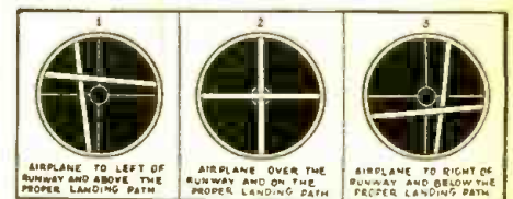
Figure 2.—The dial of the "combined instrument" with the needle pointers in three different positions.
