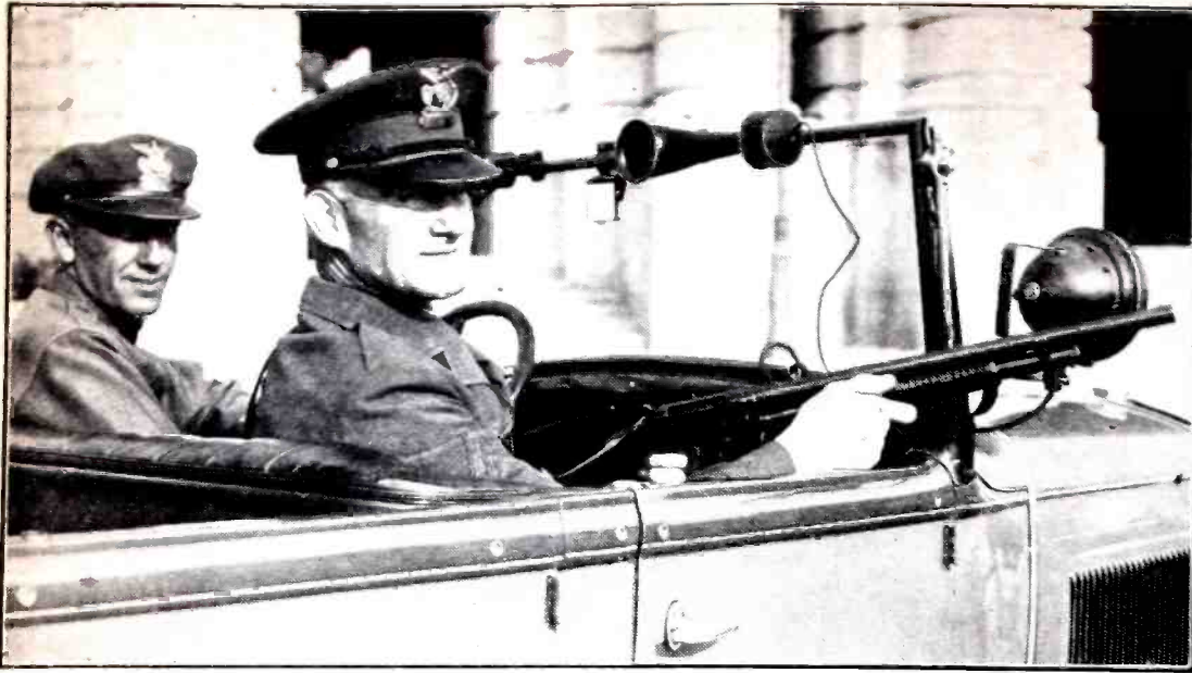
Two Los Angeles officers of the law ready for business—note the loud speaker mounted on the wind shield and which connects with a short-wave receiver.
