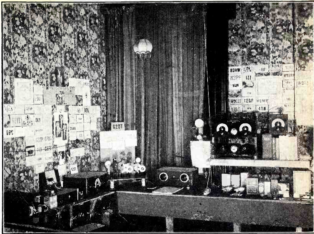
Mr. E. T. Somerset, English short wave amateur, operates this station G2DT, and experiments with wavelengths as low as 5 meters. Left to right—5 meter receiver; G.R. frequency meter type 558-P; full dial spread 9 to 90m receiver; 20 meter Hartley HI-L transmitter; frequency monitor; 40 meter Hartley transmitter; 5 meter transmitter (not visible in photo); M-L dynamotor; D.C. power supply.
