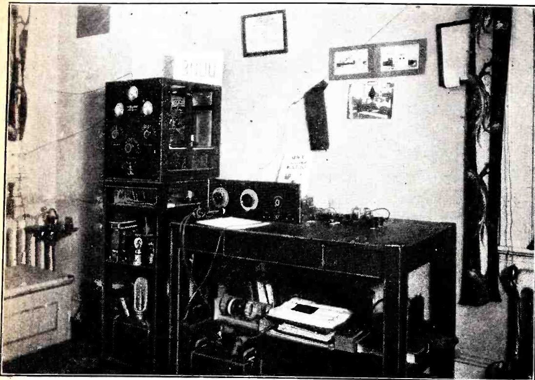
Miss Zandonini's transmitter is a 50-watt Hartley, with mercury arc rectifier; receiver employs detector and 2 stages of A.F.
