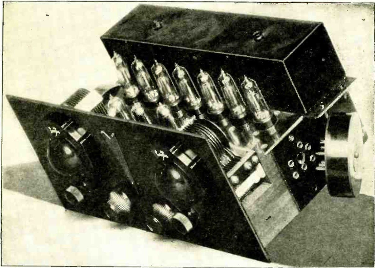
Appearance of the "Mercury" 10-tube short-wave super-heterodyne receiver.
