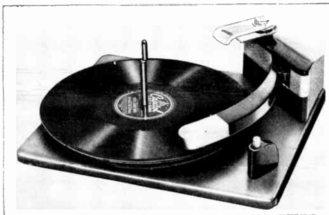
Fig. 27. A record changer with an eccentric-type spindle drop. (Westinghouse photo)
