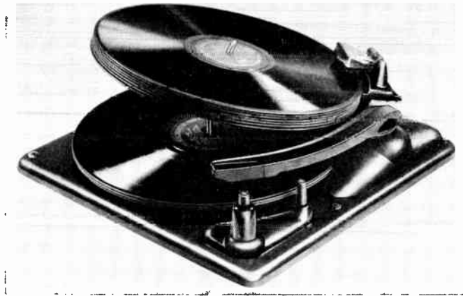
Fig. 11. A pusher or shelf-and-spindle type of record support. A pushing motion by the shelf causes the bottom record to drop down the spindle. (Westinghouse photo)
