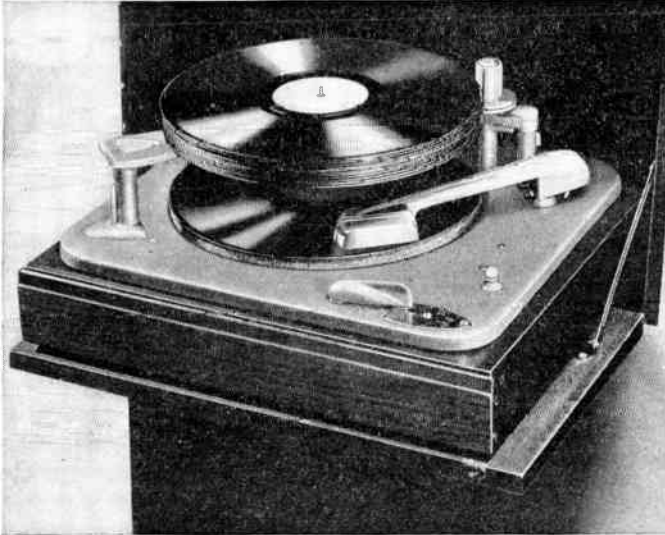
Fig. 8. A slicer-type changer with one fixed shelf and a selector shelf adjacent to the pickup arm
