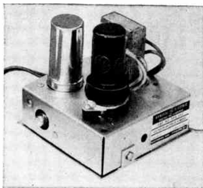
Fig. 5. A supplementary preamplifier chassis used with a regular amplifier when a GE variable-reluctance pickup is used. Low-frequency compensation is included consisting of R1, R2, and C1. (GE photo)
