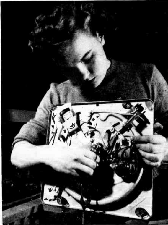
Fig. 1. Record-changer repairing is light, clean work generally requiring only adjustment of a screw or bending a piece of thin metal
