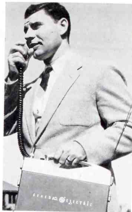
FIG. 1: NEWLY DEVELOPED PORTABLE transceiver, shown in use above, utilizes mobile industry's first transistorized receiver.
