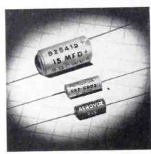
MINIATURE ELECTROLYTICS: Typical miniaturized electrolytic. Center Pee-wee in hermetically-sealed can.
