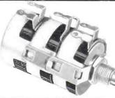
T-Pad. 11/8" Diameter. 13/4" depth from mounting surface. Impedance values from 4 ohm to 500 ohm.
