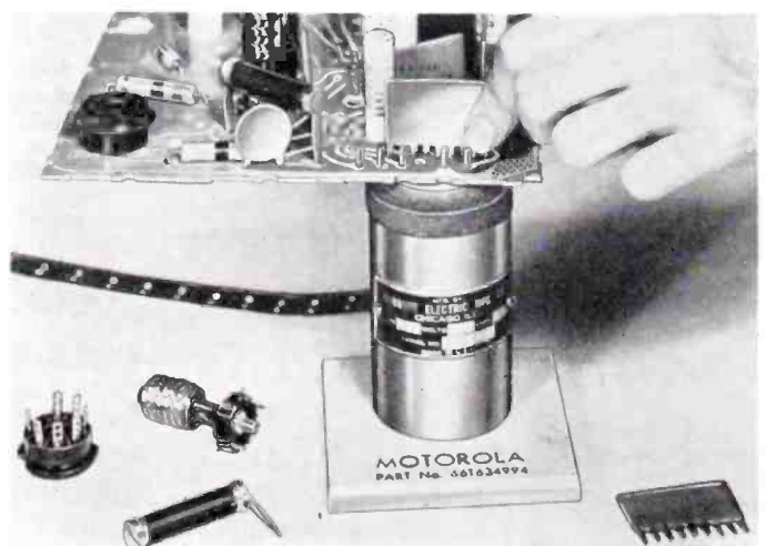
TEMPERATURE-CONTROLLED soldering pot designed to remove multi-connector component in a printed-wiring board chassis.
