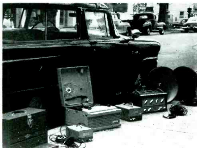
ASSORTMENT of amps, speakers, mike, recorder-playback and accessories required for effective sound-truck work.
