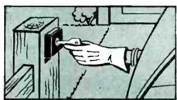
KEY-LOCK CONTROL operates from driver-level box.
