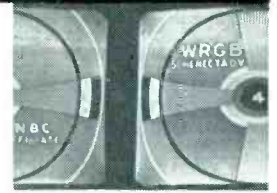
FAULT - Split picture.
