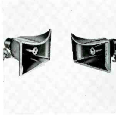
Wide-angle paging and talk-back speakers with a reflexed cobra air column for wide-angle horizontal dispersion of sound. One model has a built-in hermetically sealed driver unit integrally assembled to a reflex air column terminating in a cobra shaped wide angle bell. Cobra bell is a one-piece mold of fiberglass reinforced polyester resin. Driver unit employs a rim-centered linen-base one-piece molded phenolic diaphragm. Second model is of similar construction except that a screw-in driver unit with 7/8"-18 screw thread is used. (Models CIB [12 watts] and CMI [3 watts]; University Loudspeakers, Inc., 80 South Kensico Ave., White Plains, N. Y.)
