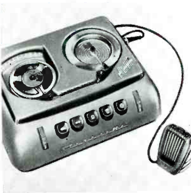
Push-button tape machine designed for 30 minutes of dictation-recording and transcribing. Five push-buttons provide control of recording, listening, forward and reverse speed winding, and stopping. Dictation corrections or playback are facilitated by automatic scale indicator. Microphone-speaker is equipped with a start-stop button to control the tape during pauses or interruptions while dictating. (Stenorette; DeJur-Amsco Corp., 45-01 Northern Blvd., L.I.C., N. Y.)
