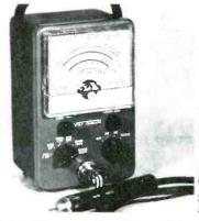
VTVM with automatic range switching said to eliminate manual selection of appropriate voltage or resistance range before use. Seven ac and da ranges of 1.5, 5, 15, 50, 150, 500 and 1,500 v; seven peak-to-peak ranges of 4, 14, 40, 140, 400, 1,400 and 4,000 v; and ohmmeter ranges of X1, X10, X100, X1,000, X10K and X100K. Features 4½" meter, 11-megohm input resistance (33 megohms on 1,500 v range). (Volt-Ohmatic; Bergen Labs, 11 Godwin Ave., Fair Lawn, N. J.)
