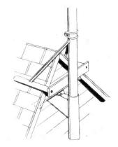
Gable mount designed for gable roofs. Accommodates tubing up to 1½" in diameter.
