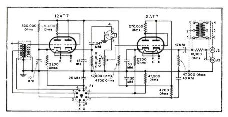
Fig. 1. Schematic of Stromberg-Carlson AV-52 preamp with a pair of twin triodes that serve as voltage amplifiers and cathode followers.
