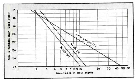
Fig. 1. Plot of axial length, height and width of a horn antenna in relation to gain achieved.
