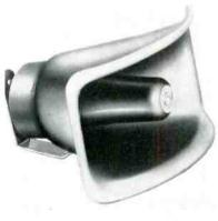
Five-watt cobra-jector speaker said to provide wide angle of dispersion in areas of high noise level, adverse wind conditions, etc. Main flare has fiberglass construction. Can be used for paging, talk-back, intercomm. industrial, marine and mobile applications. (Model CI-14. Atlas Sound Corp., 145 39 St., Brooklyn 18. N. Y.)
