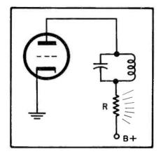
Fig. 2. Circuit illustrating point that one should never use resistors above voltage even though actual wattage is not exceeded. R (load) = .1  $\,\mathrm{w}$  and resistor rating = 1  $\,\mathrm{w}$ , but voltage across R = 350  $\,\mathrm{v}$  and voltage rating of R = 250  $\,\mathrm{v}$ ; hence resistor R will break down to over-voltage.
