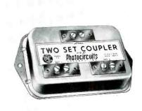
Two-set pc coupler, using wound sections of copper ribbon wire on a fiberglas support, connected to match 300-ohm signal input. (Photocircuits Corp., Glen Cove,  $\frac{N}{N}$  V.)
