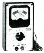
Battery tester (kit or factory-wired) for checking portable radio and hearing-aid batteries under operating conditions. Uses rotary selector switch which inserts proper dropping and shunt resistors in meter circuit to reduce terminal voltage. For 1.5 to 90 v. (Model 584; Electronic Instrument Co., Inc., 84 Withers St., Brooklyn 11, N. Y).
