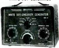
White dot linearity generator for black-and-white or color-TV. Features large and small dots for color recoiver convergence and vertical and horizontal bars for sweep circuit alignment. Internally generated vertical sync pulses are locked to line frequency for stable operation. Has ricarrier output and external modulation. (Model 160; Winston Electronics, Inc., 4312 Main St., Philadelphia 27, Pa.)
