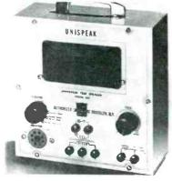
Universal test speaker designed to eliminate removal of speaker from cabinet when chassis is taken to shop for repair. Accommodates single-ended or push-pull transformers, and direct voice coil outputs; universal transformer allows impedance matching of most tubes. Includes choke and variable bleeder for matching electrodynamic speakers. Features socket and adaptor cable for plugging into the speaker or set. (Unispeak: Authorized Manufacturing Co., 919 Wyckoff Ave., Brooklyn 27, N. Y.)
