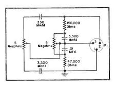
Fig. 2. Tone control developed for use with Fig. 1 preamp; Stromberg-Carlson AK-11.
