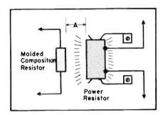
Fig. 6. Drawing illustrating need for keeping molded resistors far enough away from heat-producing components to hold ambient temperature of molded resistor below surrounding temperature, thus preventing over-
