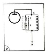
Fig. 5 (below). Gain control in video if circuit: if R is replaced with a wire-wound resistor, circuit AB shown in (a) is changed and characteristics of circuit are radically altered as noted in (b) above. (See Fig. 8 for schematic of this portion of circuit in a typical TV chassis; Coronado 15TV4.)
