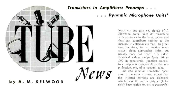
As AN AMPLIFYING device, the transistor offers many features. It is nonmicrophonic, mechanically rugged, can be operated in any position and makes extremely efficient use of its dc power supply. Transistors can oscillate with only a few microwatts of dc input
