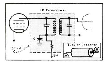
Fig. 1. Opening or shorting of capacitor C inside of an if transformer shield can is α common cause of intermittent operation. Poor connection at point A in capacitor can cause intermittent operation.
