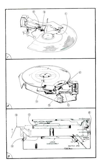
turntable to the trip lever. As a result the reject lever (coupled to the trip lever) is actuated and the latch, holding the upper subassembly in the up position, is released.
