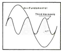
Fig. 4. In a square wave, phase relations are as important as the frequencies of the harmonics. An undistorted square wave displays harmonics going through zero at the same time as the fundamental goes through zero. If the 'scope amplifier shifts the phase of the harmonics, with respect to the fundamental, the reproduced square wave will show tilt.
