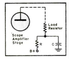
Fig. 10. Tilt, as seen in Fig. 5 (p. 21) can be compensated, and the 60-cycle squarewave response of the 'scope brought to the point shown in Fig. 2 (top—p. 20) by suitable adjustment of the values of R and C, the compensating resistance and capacitance in the 'scope-input stage.
