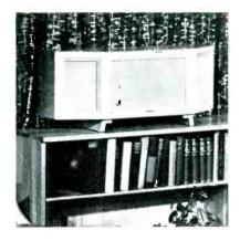
Three-way loudspeaker system with two tapered horn ports which load a coax-type low-frequency and mid-range reproducer from 70 to 3500 cps; very-high-frequency tweeter said to take over at 3500 cps to beyond audibility. Low-frequency and mid-range reproducer employs E-V Radax principle; large cone reproduces the lower frequencies and mechanical crossover is made to a smaller cone operating from approximately 1500 cps upwards. (Skylark; Electro-Voice, Inc., Buchanan, Mich.)
