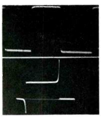
Fig. 2. Plot (top) illustrates satisfactory reproduction of a 60-cycle square wave by the vertical (video-frequency) amplifier in a service 'scope. Improper compensation of vertical amplifier causes overshoot distortion in reproduced 60-cycle square wave, as shown in bottom pattern.
