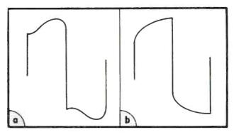
Fig. 8. Two typical examples of incorrect values of R and C in the low-frequency compensating circuit of the 'scope amplifier. When both R and C are properly chosen, the top of the reproduced square wave will be quite flat, and will exhibit
