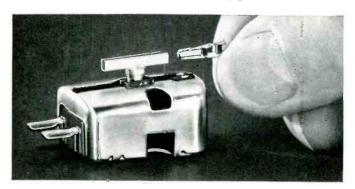
New single styli have this feature, too. Just raise the stylus shaft . . . replace the insert. A CLIP-IN TIP can be used in existing G-E dual cartridges or new single and dual types.
