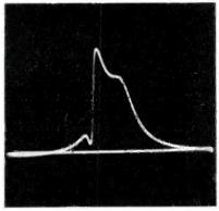
Fig. 1. A typical TV receiver response curve. This curve is most closely related to a 60-cycle square wave. If the vertical amplifier in the 'scope will reproduce a 60-cycle square wave without distortion, it will reproduce a visual-response curve without distortion. But to do this, the 'scope must respond to frequencies far below 60 cycles.
