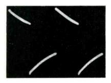
Fig. 5. Tilt in a reproduced 60-cycle square wave, due to shift in phase of the har-monics. A 'scope amplifier often shows this type of distortion, unless properly compensated. (From the Technician's Timesaver.)
