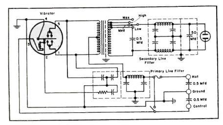
Fig. 1. Schematic of a 6-volt dc inverter. (ATR type 12, model RSE.)
