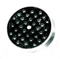
High impedance crystal tweeter that can be incorporated into plate circuit of output tube for wide-range response. Blocking capacitor in tweeter circuit is said to attenuate effectively the lower frequencies; frequency correction is in the form of a damping network tuned to resonant frequency of crystal, which damps resonance without decreasing sensitivity at other frequencies, is built into unit. Filter is an acoustic network. (Ronette Acoustical 135 Front St., N. Y. 5, N. Y.)
