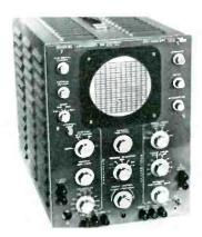
AC 'scope for 5 cps to 10 mc. Sweep circuits provide triggered or recurrent sweeps from 0.1 to 10,000 microseconds per centimeter. Internal 1-kc square wave is available for calibration and adjustment of attenuators and probes. Cathode follower outputs for external gate and sweep connections provide synchronization for auxiliary equipment. (Models 701 and 701-D; Browning Laboratories, Inc., 750 Main St., Winchester, Mass.)
