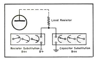
Fig. 7. Resistor-capacitor substitution box setup.
