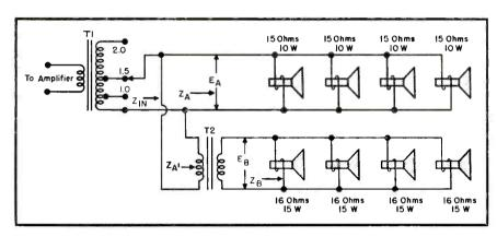
Fig. 1. An audio-system problem where we are concerned with the power and impedance requirements of different loudspeakers when operated from a single amplifier source. Specifically quirements of different loudspeakers when operated from a single angular variable. We must determine the secondary tap that is to be used on  $T_1$  and the turns ratio of  $T_2$ . In leg A, we find that  $Z_A = 15/4 = 3.75$  ohms.  $P_A = 10 + 10 + 10 + 10 = 40$  watts.  $E_A = 12$  v.
