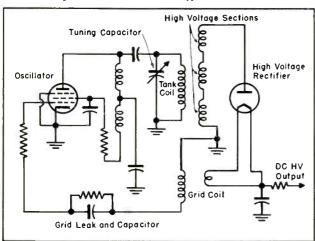
Fig. 2. Diagram of clamp type of feedback.
