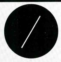
Phase shift between horizontal-vertical amplitiers, 0-100 kc-0°, to 1 mc within 2°; by internal adjustment with gain controls at max 0° phase shift possible on any specific frequency to 6 mc.
