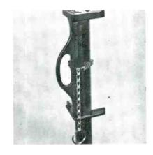
Bubble plumb for TV antenna-mast installations. Consists of two level vials mounted on right angle arms to enable operator to line any object vertically plumb. Right angle levels provide reference of all directions. Fastening devices permit attachment to objects  $\frac{1}{2}$ " up to  $\frac{1}{2}$ ", round or square. Holds itself in place. Size is  $\frac{4}{2}$ " average all-aluminum. (Clark and Newcomb, 305 Chapman St., Greenfield, Mass.)
