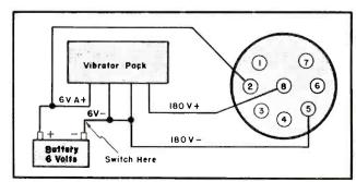
Fig. 2. Battery-operation plug and circuit.
