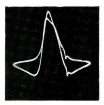
Fig. 6. If the 'scope amplifier introduces tilt into a reproduced 60-cycle square wave, it will introduce loop distortion into a reproduced response curve, as shown. Proper low-frequency compensation of the 'scope amplifier eliminates this difficulty. (From Technician's Timesaver.)
