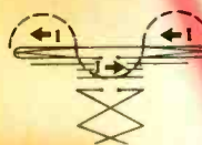
Current Distribution (Channels 7-13) Without Helix
