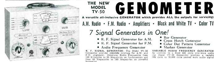
GENERATOR: The Model TV-50 projects an actual Bar Pattern on any TV Receiver Screen. Pattern will consist of 4 to 16 horizontal bars or 7 to 20 vertical bars.
