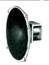
Eight-inch extended range speaker with 6.8-ounce Alnico V magnet, a power rating of 15 watts and a response up to 12,000 cps. It is equipped with an aluminum voice coil. (Model 850; G.E.)
