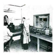
Antenna research laboratory recently set up by Ward Products Corp., in Ashtabula, Ohio, for the design and testing of TV and automotive antennas. According to W. H. Rickards, Ward director of engineering, test facilities include equipment for the measurement of impedance, vsw1 and gain. A pattern range has also been constructed in the lab.
