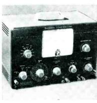
Audio analyzer said to function as three instruments in one; ac vivm, waitmeter, and intermodulation distortion analyzer. Fcatures built-in low and high-frequency osciliators. (Model AA-1 (kit); Heath Company, Benton Harbor, Mich.)
