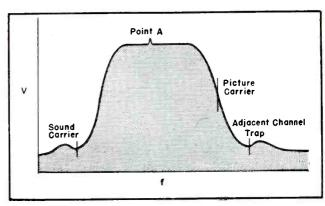
Fig. 2. Typical if response curve, with point A the carrier point of TVI as it appears in these stages.
