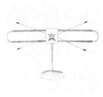
Indoor antenna designed for uhf and vhf. In areas where uhf reception only is desired, antenna can be adjusted so that the vhf dipoles serve as a reflector element for the uhf fan. Constructed of aluminum and shock-proof plastic, and supplied with 8' of 300-ohm line. (Coronet Electronics, Inc., 505 North LaSalle St., Chicago 10, Ill.)
