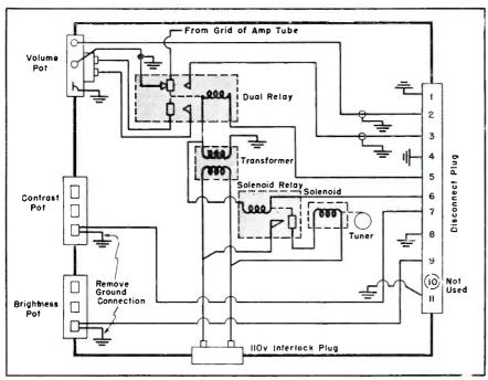
Fig. 1. Wiring diagram of TV Remot-o-matic (De Luxe system) remote.
