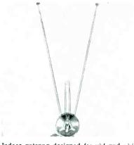
Indoor antenna designed for vhf and uhf. The uhf center section is adjustable in length allowing it to be resonated to the desired uhf channel. In other switch positions, the same adjustable center section acts as a variable stub on vhf. Effect of hand capacity is said to have been eliminated through the use of a plastic insulating knob at the top. (Model TA150; JFD Manufacturing Co., Inc.)
