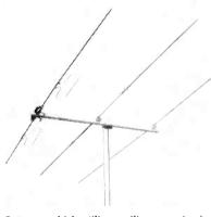
Antenna which utilizes collinear-yagi principle. Driven element with wave traps is backed by hf and If reflectors providing six working elements on the high band. Snap-lock design. Available as a single, two stocked and four stacked array. Fiberglass insulators used to isolate the antenna sections; they also provide snubbing action said to add to life of antenna. (Model 1870, Trapper, Jr., Technical Appliance Corp.)
