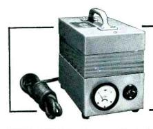
Regardless of line voltage supply, the Automatic Voltrol corrects voltage fluctuation over a range from 95 to 130 volts. The voltmeter supplied indicates secondary voltage while unit is in operation. A built-in relay automatically disconnects circuit when set is turned off.
