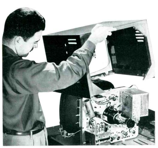
New super-vertical chassis filament circuit—employs 14 new, ruggedized 600 mil tubes . . . provides faster warm-up and far less chance of tube failure than sets using transformers. Parallel tubes and resistors are eliminated.
