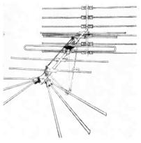
Combination conical-yagi TV antenna with radar-flector. Factory preassembled. Available in single array and 2-array models. Employs seventeen hi-tensil 3/4" aluminum elements, three perma-plastic insulators, a six-element radar-flector, plus a universal U clamp, crossarm support and 60" twin lead phasing stub. (Texas Ranger models AX673 and 674; Snyder Manufacturing Co., Phila., Pa.)
