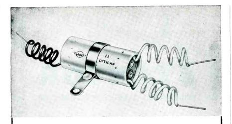
NEW DUAL SECTION ELECTROLYTIC CAPACITORS HERMETICALLY SEALED IN ALUMINUM TUBES WITH COMPLETELY FLEXIBLE INSU-LATED LEADS. By riveting the leads directly to the condenser end disc, Planet has eliminated the use of rigid terminal risers ordinarily used on this type construction. This allows Planet Type IL capacitors to fit into a smaller space and eliminates the possibility of lead breakage.
