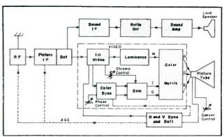
Fig. 2. Schematic of a color receiving system.
