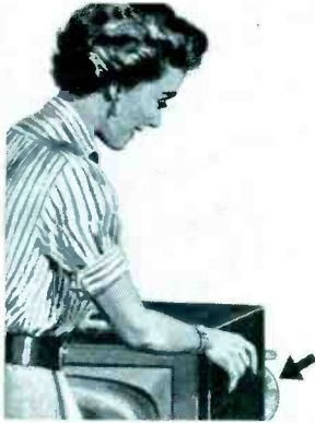
Concealed uhf all-channel converter designed to fit completely inside a TV set. All that can be seen of finished installation is a plastic selector dial and switch. Converter also offers a choice of mounting positions; at left, right or top of cabinet. (Model 188; P. R. Mallory and Co., Inc., 3029 E. Washington St., Indianapolis 6, Ind.)
