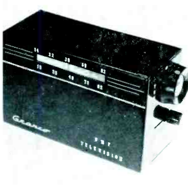
A uhf tuner developed for concealed installations; metal-cased tuner mounts at rear of TV set, and slide-rule tuning dial protrudes slightly above top, while tuning knob and selector switch are accessible at right rear. Unit incorporates coax-cavity continuous tuning over the entire uhf band and preselection. (Hiway models HT-1, HT-2 and HT-3; Granco Products, Inc., 36-17 20th Ave., L. I. C. 5, N. Y.)
