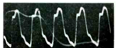
Fig. 4 (below). Another waveform obtained during a 500-kc square-wave test of the same frequency-compensated video amplifier used to obtain waveform shown in Fig. 3. This reproduced square wave exhibits high-frequency smear.
