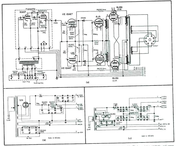
Fig. 1. Circuit of McIntosh 50-W-2 using 6Ls and 20-W-2 with 6V6s (dashed lines indicate change in circuit, with 470-ohm resistors omitted): and power supplies for each amplifier. Input and output plug connections provide assorted impedance matching for 4 to 600-ohm requirements.
