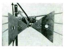
A uhf antenna adaptor; an all-channel. uhftriangular dipole. A preassembled unit, it can be fastened to the front end of super fam. The distance is said to be pre-fixed, and the uhfdipole is veed forward so that it is always parallel to the vhf fan elements which function as a sheet reflector. Designed for use with separate vhf and uhf leads to TV set or con-verter. (Model 415, Econo-Dapter; Channel Master.)
