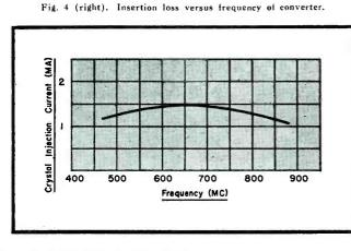
Fig. 3 (below). Plot of injection current versus frequency.
