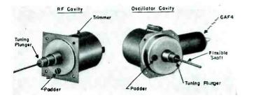
(Above) Fig. 5. View of tuning elements used in coax unit.
