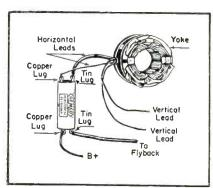
Fig. 5. Circuit ilustrating installation of horizontal reframer. Fig. 5a. Three types of horizontal reframers available to compensate for low line voltage which can lead to horizontal shrinkage. (Courtesy Gemco)
