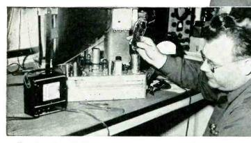
**1. ISOLATING THE TROUBLE**—Plug the power cord of the chassis into LOADCHEK and note the reading. With your eye on the large meter remove the rectifier tube and you can tell immediately which side of the tube the trouble is on. You have already eliminated 50% of your probing time.
