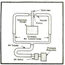
a hole in the sample. The nozzles on the end of the air column are adjusted for a small clearance and the air supply is turned on. The test part vibrates at its resonant frequency and the air column is tuned to give a maximum vibration displacement.
