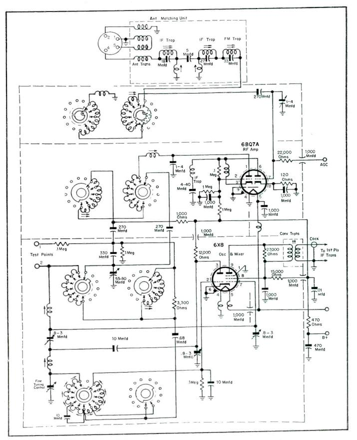
coupled circuit is determined by the coupling capacitance and the crystal loading. (Crystal loading is determined by the crystal tap point on the secondary and the oscillator injection current to the crystal.)
