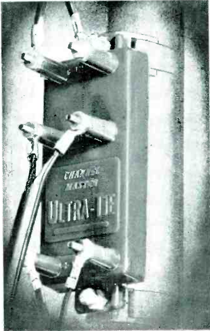
Interaction filter designed to combine separate antennas into a single vhf/uhf system for one-lead use; see p. 78 for details. (Courtesy Channel Master)
