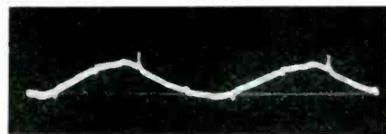
Fig. 4. A small series capacitor in a crystal probe serves to attenuate 60-cycle heater voltage to a very small value, and provide this display; at the same time, if there are harmonics in the heater voltage, these harmonics will be relatively enhanced. Here is a case where the harmonics of the heater voltage are feeding through a crystal probe. Service Men must avoid confusing such harmonics with demodulated spurious rf voltages. In case of doubt, the rf and if tubes should be removed to determine whether the display is changed.
