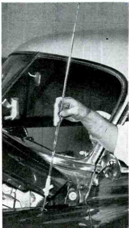
How antenna assembly can be mounted from the top of the fender or cowl.
