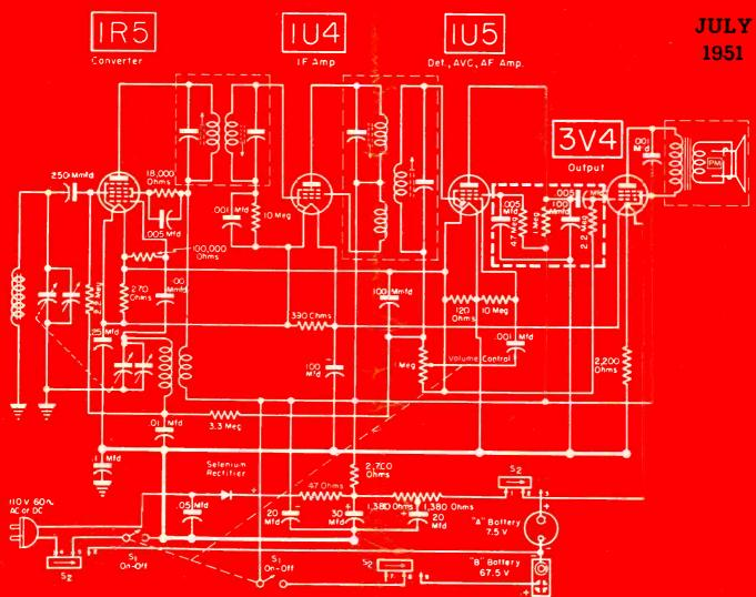
Four-tube ac-do-battery portable featuring a printed-circuit audio-coepling assembly.
