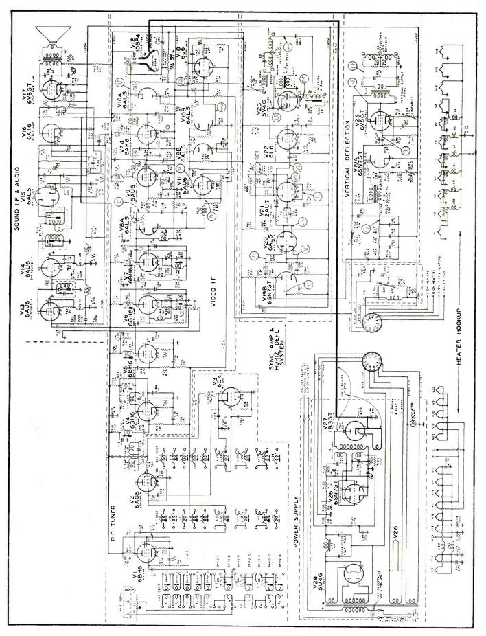
stages using 6BH6s. At the output of the third 6BH6 pix stage, sound energy is taken off by means of  $L_m$ , the
