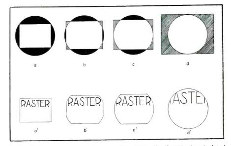
Fig. 1. Viewing areas most commonly seen on picture tubes. The illustration in a is that of the viewing screen on monitor equipment, while in b, c, and d appear the viewing areas on typical commercial TV receivers. In a', b', c' and d' appear the effects on the picture in each of the four types of areas illustrated in a, b, c and d.
