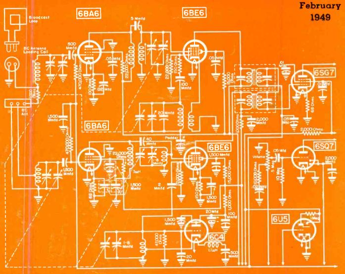
The rf, converter, mixer, oscillator, if, first of and tuning indicator stages of a 10-tube AM/FM tuner. [See page 2] THE TECHNICAL JOURNAL OF THE RADIO TRADE
