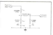
Fig. 1. Alternate If compensation circuit.
