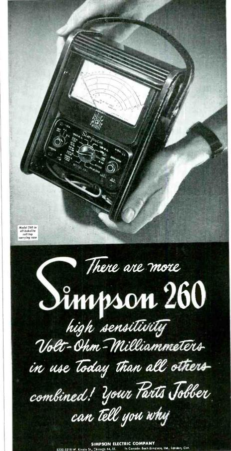
RANGES at 20,000 ohms per volt DC, 1000 ohms per volt AC VOLTS: AC & DC-2.5, 0, 50, 250, 1,000, 5,000 DC CURRENT: 10, 100, 200 MA-10 AMP-100 MICRO AMP OHMS: 0-2,000 (12 certer), 0-200,000 (1200 center), C-20 MEGOHMS (120,000 ohms center) DECIBELS: (5 ranges) -10 to +22 DE
