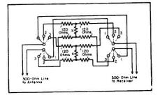
Fig. 3. A two-gang double-pole three-position selector-switch arrangement which permits insertion of pads in 300-ohm lines in those channels where the TV signals are too strong.
