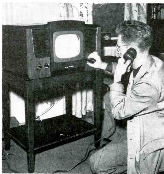
Relaying antenna-position instruction via a sound powered phone in the home. (Courtesy RCA.)
