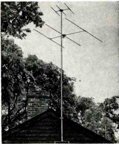
Fig. 6. A double stack of three element arrays, which serves to increase the forward gain of a specific tv channel. (Courtesy Workshop Associates)
