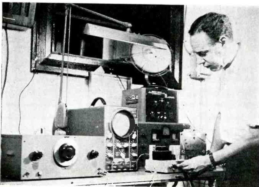
Checking vibrator power supply with a 'scope.
