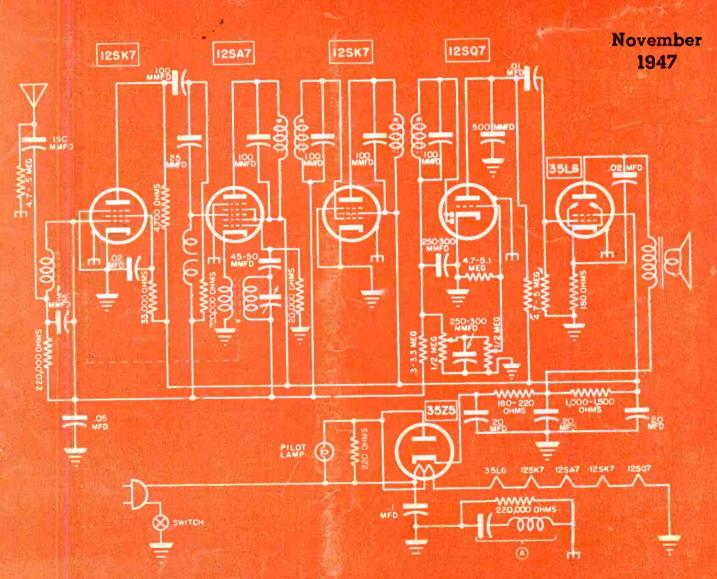
Five-tube a-c/d-c receiver, with slug-tuned i-f's, developed for coin-operated usq. [See page 2]
