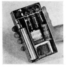
Standard type volt-ohm-milliameter may be plugged into jacks so that the unit may be used as an effective r-f vacuum tube voltmeter...
