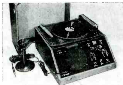
A dual speed recorder permitting recording of 12 minutes on a 10" disc at 33½ rpm and copying of a 12" commercial record on a 10" blank at 78 rpm. (Courtesy Bell Sound Systems)
