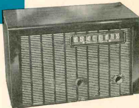
COMPANION MODEL No. 571. 5 Tubes. AC-DC. Superheterodyne Circuit. Built-in Antenna. Automatic Volume Control. 2-Gang Air Condenser Tuning. Illuminated Slide-Rule Dial. Standard American Broadcasts. Walnut Veneer All-Wood Table Cabinet, 13 \frac{1}{8} " x 7 \frac{1}{8} " x 8 \frac{3}{8} ".
