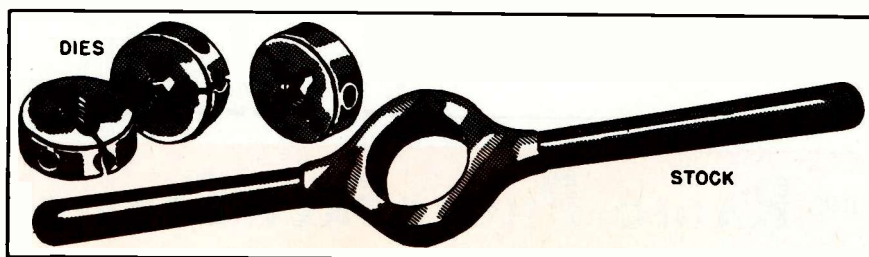
Fig. 4. A small stock and several removable dies of different sizes that fit into it. These are useful for threading rods or cleaning up damaged threads or screws.
