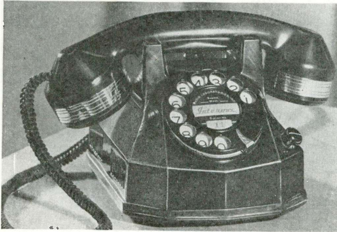
Fig. 1. View of dial-controlled intercommunications unit.
