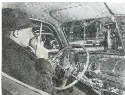
Two-way radiotelephone-equipped police car using recently developed Kellogg coiled kord. (Courtesy Galvin Manufacturing)
