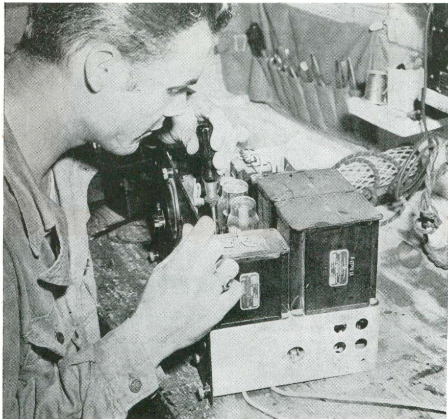
Fig. 1. Using screwdrivers in servicing. Since screwdrivers are the most often-used tools in the Service Shop, they should be chosen very carefully. (Courtesy U. S. Army Signal Corps.)
